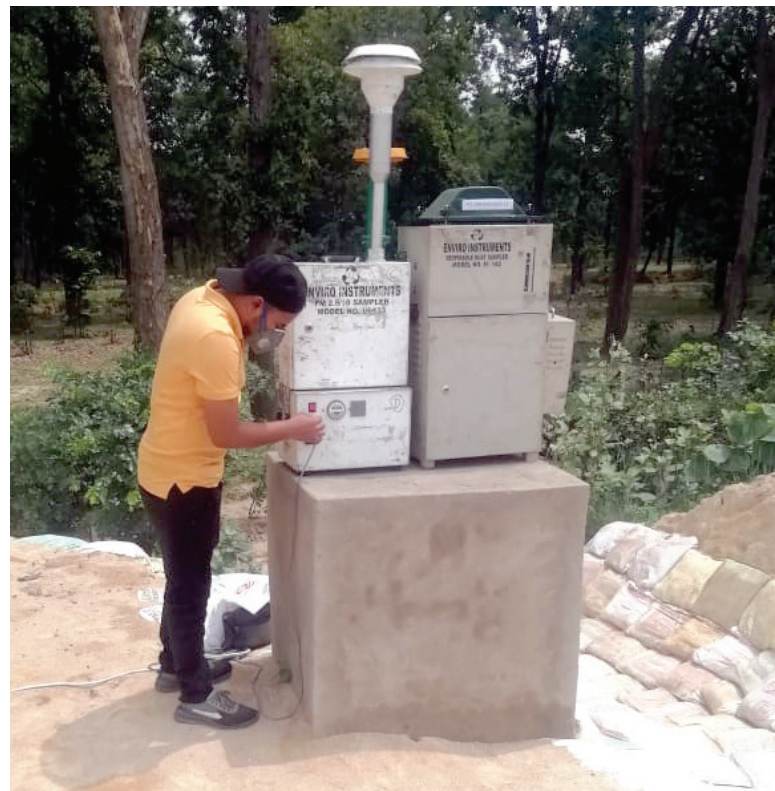
Sampling of PM_{10} and PM_{2.5} in dust emission
